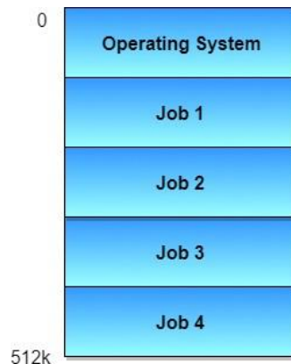
Figure: Memory layout for a multiprogramming system.
