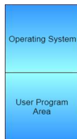
Figure: Memory layout for a simple batch system
